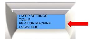
①. Using the arrow keys , select "RE-ALIGN RED POINTER" and validate .
